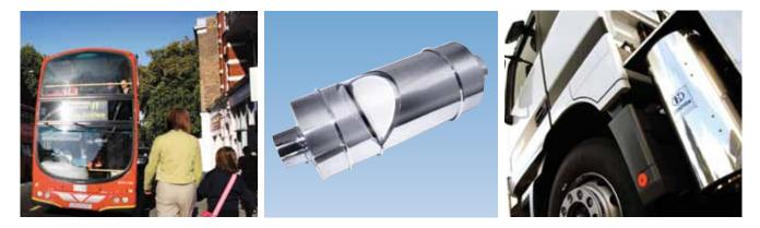
The Eminox CRT® system is Europe's leading diesel particulate filter, with around 60,000 systems installed on buses and trucks worldwide. Our CRT system reduces Particulate Matter (PM) emissions by more than 90%, allowing vehicles as old as Euro I to be upgraded to the PM standards of a Euro IV vehicle.
