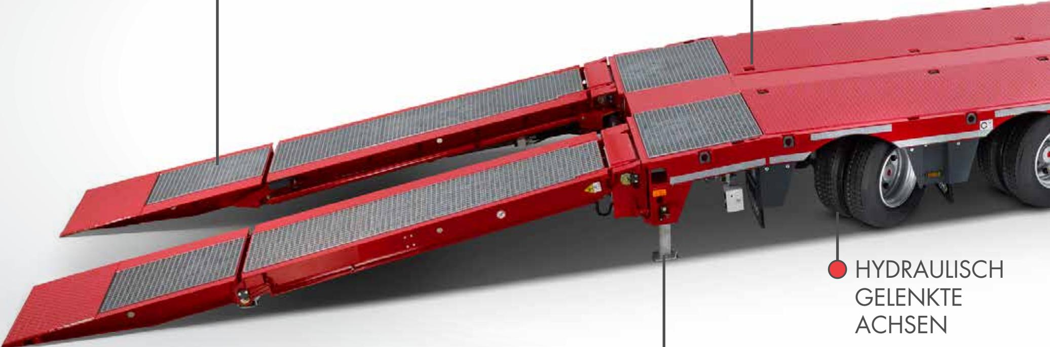
● HYDRAULISCH FALTBARE AUFFAHRAMPEN
